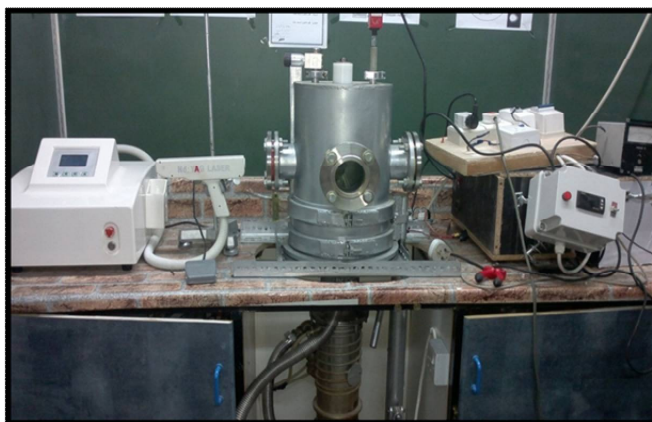
Fig.(1): Pulsed laser deposition (PLD) system.
